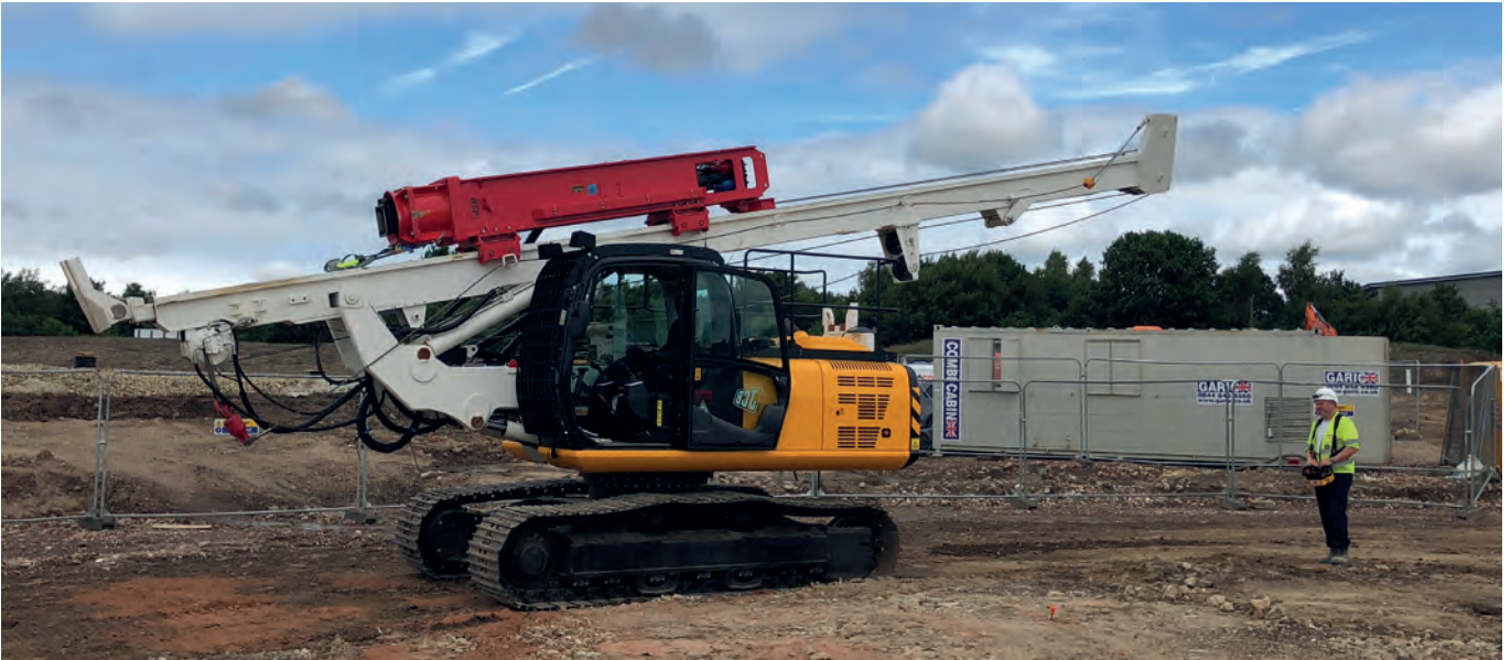
RIG BEING OPERATED BY RADIO CONTROL
