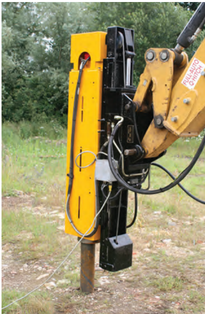
BH120 DRIVING STEEL PILES
