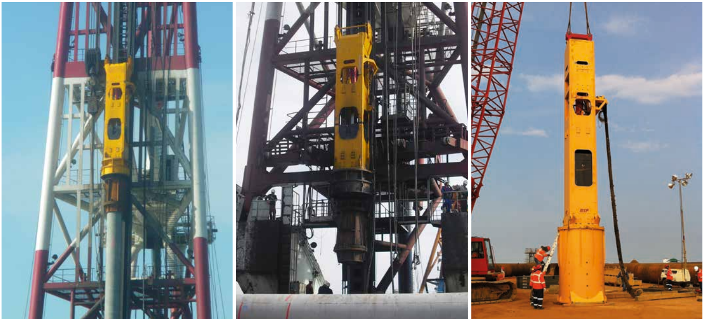
ABOVE: HAMMERS SHOWN IN LEADER MOUNTED OPERATION. CRANE SUSPENDED OPTION ALSO AVAILABLE.
